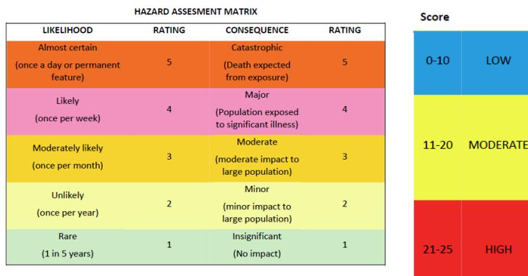
**Figure 2: Risk matrix used for the W<sub>2</sub>RAP tool**
